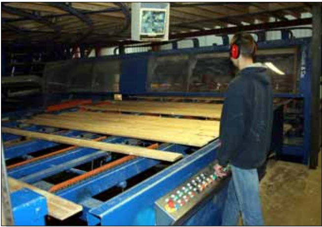
Building the layer before cross-cutting
