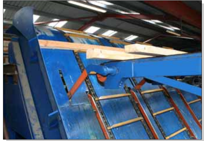
Tiltable waterfall singulator is receiving main product from upper conveyor and sideboards on the lower
