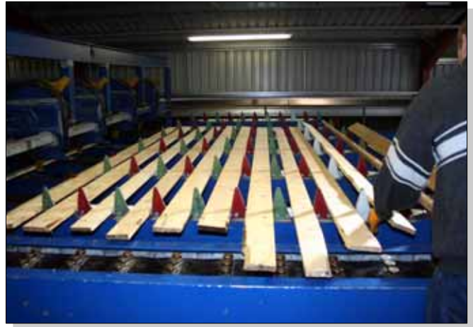
Boards are inspected on shark fin turner
