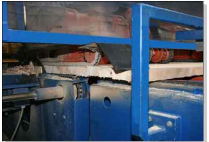
Boards are trimmed and cross-cut
