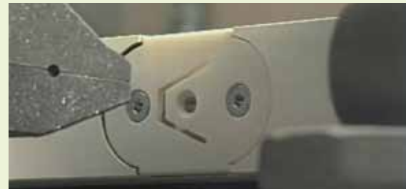
A hinge is mounted and fastened with screws. All this takes place in one fully automated operation.
